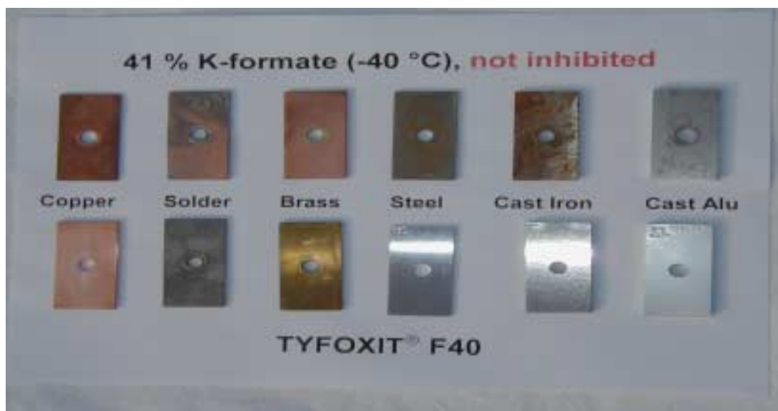
F6: Appearance of Metal Specimens after Corrosion Test acc. ASTM D 1384
